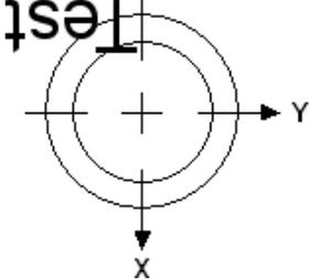
Note that the text moved up relative to the calibrated center of the laser presenter's nozzle because the value of Y is negative. Therefore for positive values of Y, the text will move down from the calibrated center of the laser presenter's nozzle.
