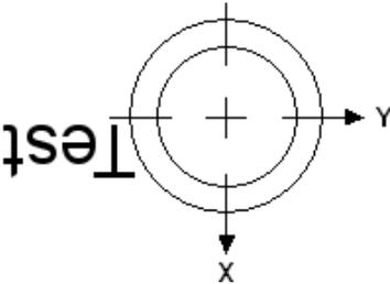
Note that the text moved left relative to the calibrated center of the laser presenter's nozzle because the value of X is positive. Therefore for negative values of X, the text will move right from the calibrated center of the laser presenter's nozzle.
