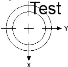
Note that the text moved up relative to the calibrated center of the laser presenter's nozzle because the value for Y is negative. Therefore for positive values of Y, the text will move down from the calibrated center of the laser presenter's nozzle.
