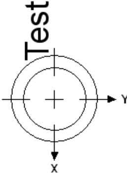
Note that the text moved up relative to the calibrated center of the laser presenter's nozzle because the value of Y is negative. Therefore for negative values of Y, the text will move down from the calibrated center of the laser presenter's nozzle.
