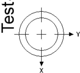
Note that the text moved left relative to the calibrated center of the laser presenter's nozzle because the value of X is positive. Therefore for negative values of X, the text will move right from the calibrated center of the laser presenter's nozzle.
