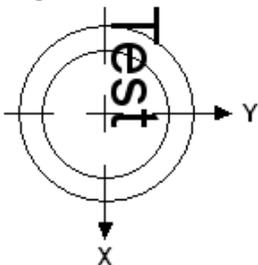
Note that the text moved up relative to the calibrated center of the laser presenter's nozzle because the value for Y is negative. Therefore for positive values of Y, the text will move down from the calibrated center of the laser presenter's nozzle.
