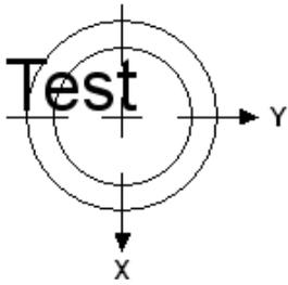
Note that the text moved left relative to the calibrated center of the laser presenter's nozzle because the value for X is positive. Therefore for negative values of X, the text will move right from the calibrated center of the laser presenter's nozzle.
